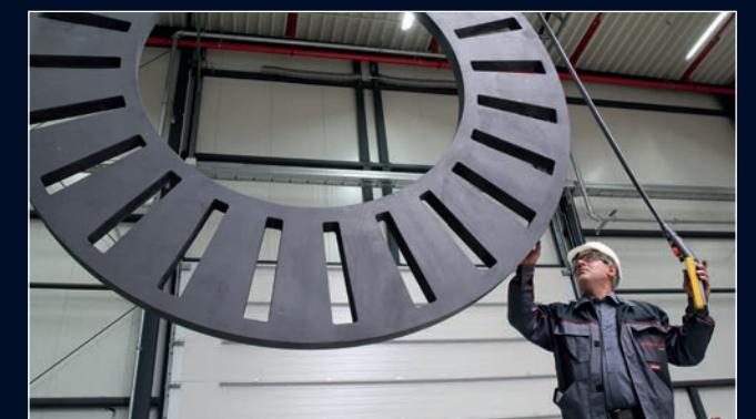
Distributor plates from KERA® 21 for a production plant for white phosphoric acid.
