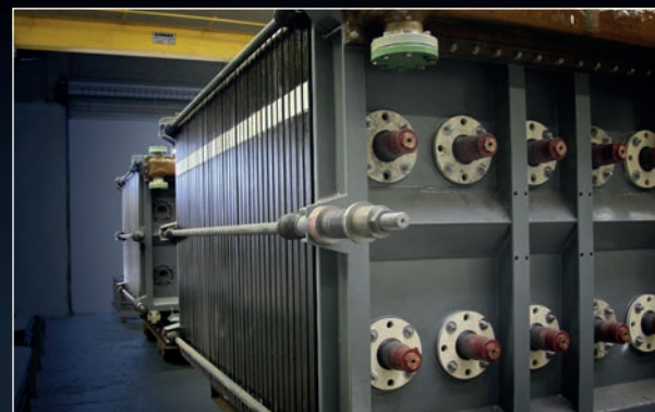
Hydrochloric acid (HCl) is separated during electrolysis with KERA® frames into chlorine gas and hydrogen.
