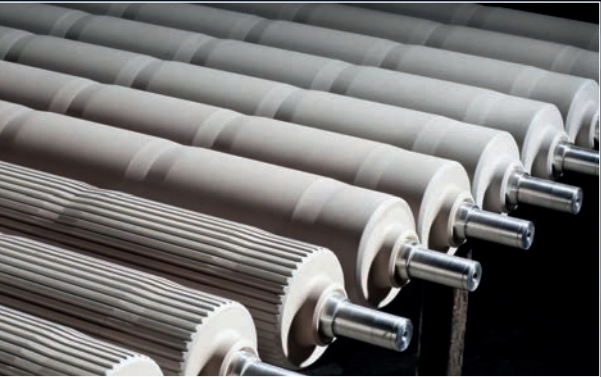
Rollers made from KERA® SP 20 used for cellulose processing, with 20 % sulphuric acid (H 2 SO 4 ) as the process medium and a working temperature of 70 °C.
