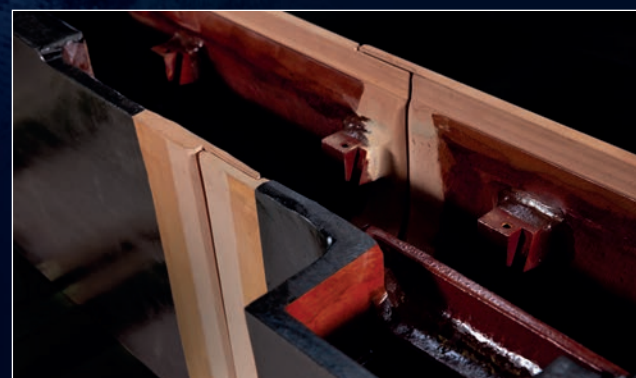
Sulphuric acid process vessel made from KERA® SP 20 in the viscose fibre industry. The many individual segments are precisely assembled and securely bonded together on site.
