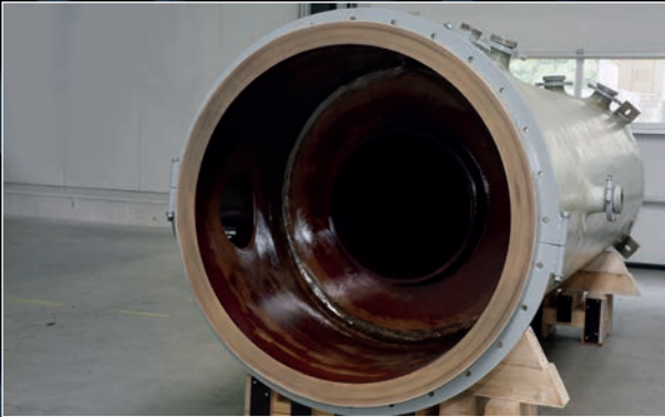
Complete HCl absorber made from KERA® SP 30 / FRP for extreme operating environments. In this case, 32 % hydrochloric acid (HCl), operating temperatures of up to 120 °C, designed for an operating pressure of -1.0 / + 0.5 bar.
